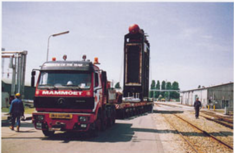
Dordrecht — A 140 tonne furnace with accessories was transported for a major extension of a Dupont petrochemical plant in Dordrecht. Somewhere else on the site a 90 tonne reactor column was erected and positioned.
