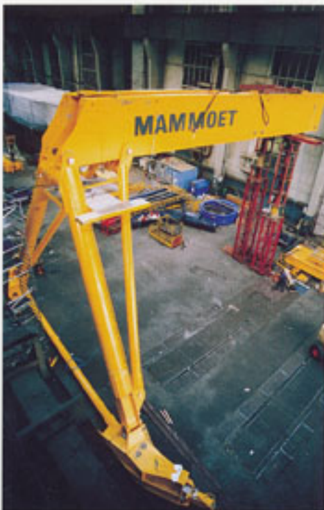
Rotterdam — This temporary lifting device was built by Huisman Itrec. The various parts were assembled in Rotterdam before shipment in order to check the system on teething problems. Thereafter the gantry was dismantled and made ready for shipment to the U.S.A. There it will be used in a lifting set-up with Mammoet's HydraJack lifting system for the exchange of steam generators in nuclear power plants.
